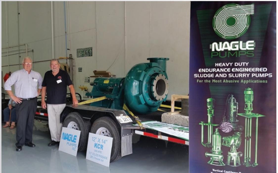
Bill and Tim Triplett display the KCR pump at an industrial show hosted by Process and Power Distributors. This 12" x 14" pump will be used for "white water" which is a mixture of mineral wool and perlite used in the manufacture of ceiling tile at Armstrong World Industries. The impeller will allow passage an 8" solid and it runs at a very slow speed 400 to 500 rpm.
