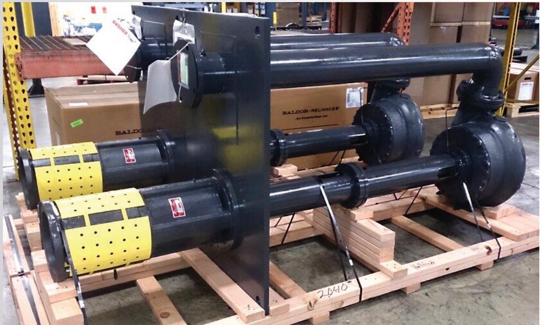
Mike Jones sends these...a couple of nice vertical pumps. These are Gusher V6X8 -15 - VSEL +47-CDM-A-DP, 73 7/8" long, rated at 1500 GPM at 43 TDH , driven by 60 HP at 1800 RPM motors, going into the Honda CAPT plant pumping coolant and chips back to a coolant filtration system
