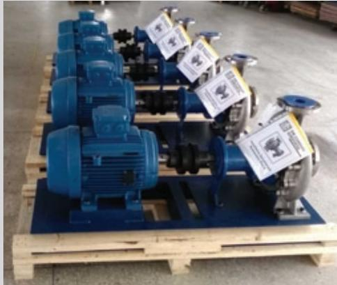
Gusher Shanghai sends photos of a recent DIN pump project. Entirely manufactured in China, these 5 model 80/315 model Din pumps are constructed in 316 stainless steel and include Chinese made 18.5 kw WEG motors. This is the first order of its kind for Gusher's China division.
