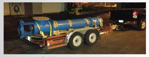
Loaded and ready for delivery to a new customer in Louisiana, is a Deming Mixed Flow Pump with a 18" fabricated discharge head rated for 9000 GPM at 40' TDH.
