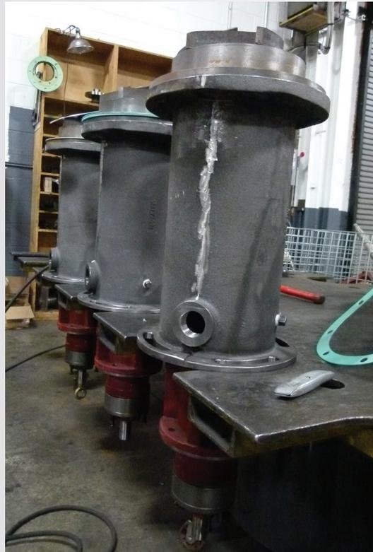
*Shown here are Three 3 x 4 x 10B Enclosed Column Pumps ready for finishing..*
