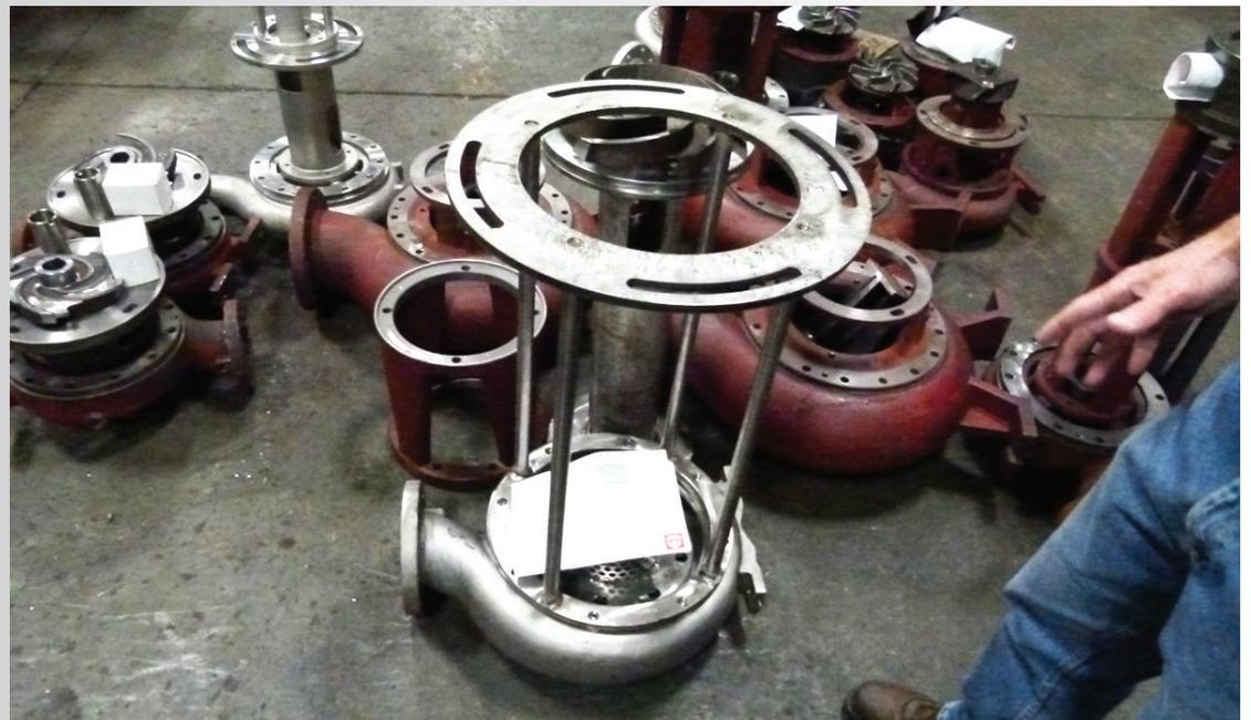
*Assembly parts for a 4 x 6 x 13 Top Pull Out 7600*
