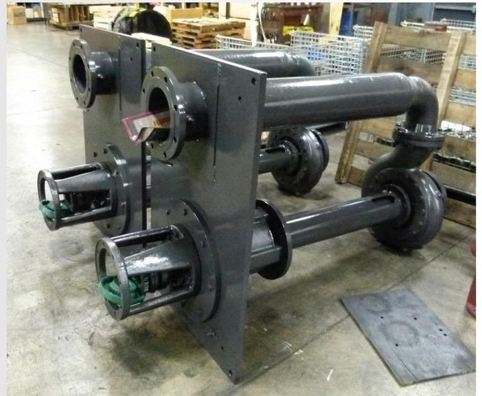
*Tim Keetor shown here working on one of two Giants. These 7550 Vortex Pumps are 75 HP, 1600 GPM and designed for an 88 inch immersion depth. These will be going back to the Dry Ridge facility for a customer witness test for a Great Lakes Pump and Supply customer.*
