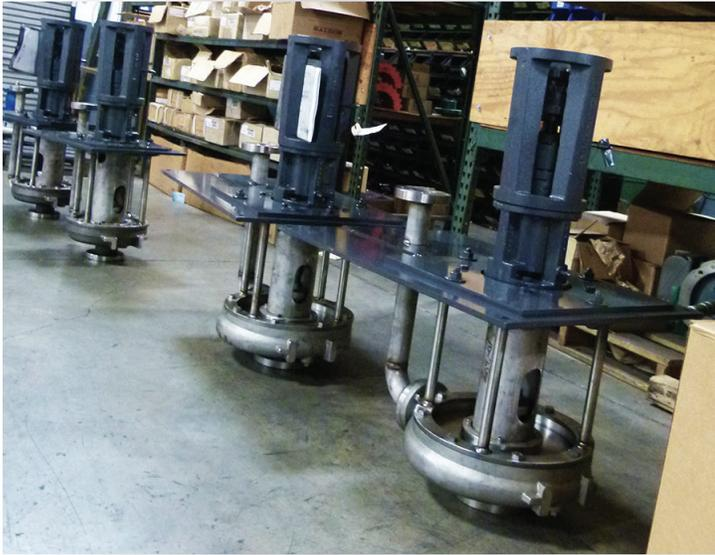
*These finished Top Pull Outs are awaiting motors. Also sold by Great Lakes Pump and Supply, these operate at 15 Hp, 45 PSI, pumping 150 GPM.*
