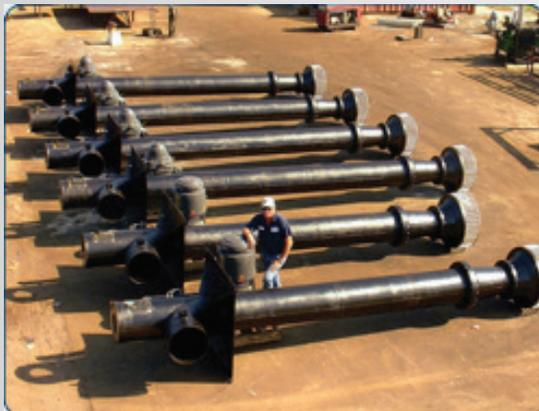
Axial Propeller Pumps
