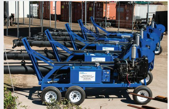
A set of hydraulic power portable pumps built for Thailand.
